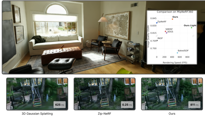
Fig. 1: RadSplat enables high-quality real-time view synthesis for large-scale house-level scenes [2] at over 900 frames per second (top). In contrast to 3D Gaussian Splatting [21], our method allows for robust synthesis of complex captures while rendering 3,000 \times faster than the state-of-the-art in offline view synthesis, Zip-NeRF [2] (bottom).
